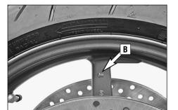
To mount, lift the front wheel in the fork and mount the wheel spindle and collar screw [2]. Tighten the collar screw to 60 Nm. Position the brake calipers and make sure the brake pads are correctly positioned. Apply Loctite 243 to the screws [1], mount the screws and tighten to 45 Nm.
