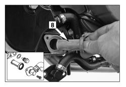
Carefully pull the oil screen [8] out of the oil tank.
