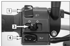
⇔ The indicator switch [3] returns to central position after actuation. Press flasher switch towards switch housing to switch off the flasher.
