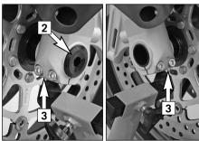
Loosen the collar screw [2] and the clamping screws [3] on both fork leg axle passages. Unscrew the collar screw approx 8 turns, press on the collar screw with your hand to push the wheel spindle out of the fork leg axle passage and remove the collar screw. Hold the front wheel while you pull out the wheel spindle. Lift the front wheel off the fork.
