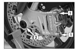
Remove the screws [1] from the left and right brake calipers and carefully pull the brake calipers off the brake disks towards the back.
